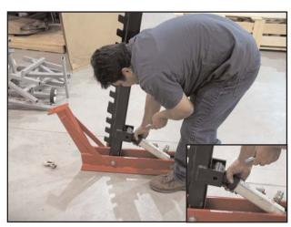
Attach ram coupler to post using supplied nut & bolt.
