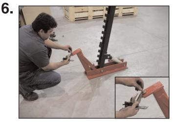
Attach hook to back of base by with supplied locking pin
