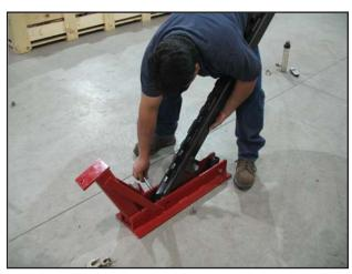
Attach post to base using supplied nut & bolt.
