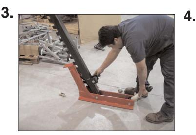
Remove bolt from ram coupler on post.c
