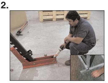
Screw hydraulic ram onto ram coupler at end of base. Hydraulic ram may or may not be included depending on which package you buy.
