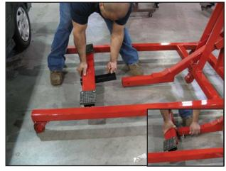
Slide the assembled adapter into the lift beam of the lift. Lock it into place with the supplied locking pin.
