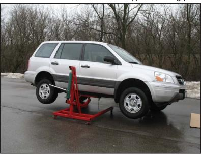
Your lift is now ready to use. Make sure that the lift pads are placed in an approved lifting section of the car. Contact the vehicle manufacturer if you are not sure where to place the lifting pads.
