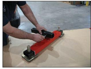
The adapter attaches to the cross beam adapter with the supplied bolt.
