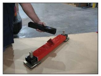
The jack beam adapter has a slot one side.
