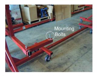
Lift vehicle and bolt vehicle frame to Frame Supports using supplied mounting bolts. Caution: Bolts are Grade 8 and should only be replaced with Grade 8 if ever damaged.
