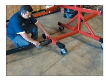
Insert Beam into Frame Supports.
