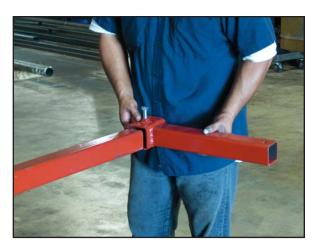
Insert Bracket Arm into Bracket Arm Support. Adjust to desired width to align with mounting holes on vehicle frame and tighten locking bolt securely.
