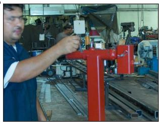
Insert locking pin to hold swivel in place
