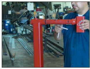
Insert Bracket Swivel into Base Mount. Applying a light layer of grease before inserting will allow for easier rotating of vehicle.
