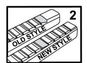
Lubricate Shaft With Light Machine Oil at BOTH ENDS Weekly
