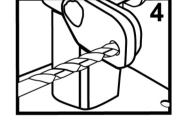
Install Shim PRIOR to Bolting Bracket Down to Make Sure it Lays Flat in bottom of tube.
