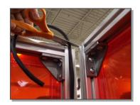
2. Unroll the 8' long corner cover and cut to the same height as the rubber welting. Discard the remaining corner cover material
