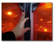
4. Starting at the top of the frame, press the round rubber welting on to the face of the corner cover material and into the vertical groove in the face of the aluminum frame until you have reached the bottom. (TIP: A squirt of "Windex" directly on to the rubber welting allows it to slide into the aluminum groove more easily).
